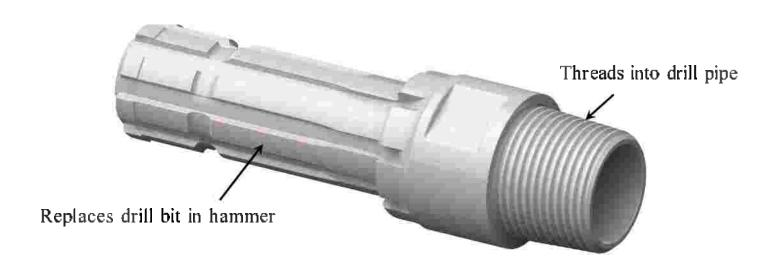
Constant hammer shanks or "Rattler bits" are used in a hammer in place of a standard drill bit and allow the pis- ton to continuously cycle when the air is turned on. They are typically used when a hammer and drill string is bogged to rattle the drill string.
